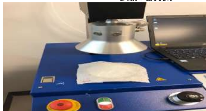
FIG:6 TSI 8130A FOR FILTRATION EFFICIENCY AND PRESSURE DROP MEASUREMENT [7] .
