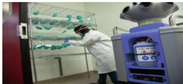
FIG:6 USING A BIOQUELL (HORSHAM, PA, USA) HYDROGEN PEROXIDE VAPOR GENERATOR, DUKE UNIVERSITY HOSPITALS STAFF CAN DISINFECT, FOR REUSE, 1250 MASKS PER CYCLE, AND 2500 PER 12 H SHIFT
